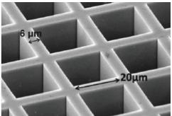
The Goddard-provided soft X-ray Wide-Field Imager proposed for a mission called ISS-TAO borrows heavily from nature. The images on the left and center show close-up views of a crustacean's eyes; the image on the right shows a manmade microchannel plate. Both operate the same way. Both gather light from multiple angles, focusing it into a single image to provide a wide field of view. Credit: J. Camp
