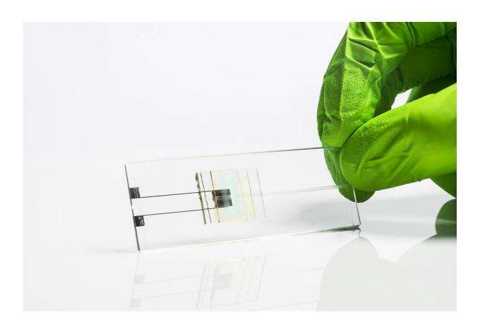
Pocket laboratory: Fraunhofer IOF's new printable fluorescence sensors hope to offer a quick and easy way to detect disease markers in the blood. Credit: Fraunhofer IOF
