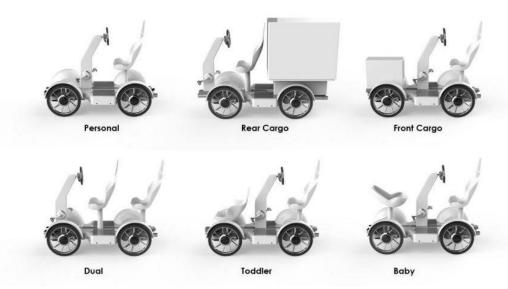
The transformative Hybrid Module Mobility design concept that can change its forms into six different modules, according to users' needs. Credit: UNIST
