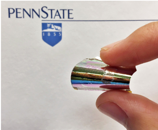
Electroded thin-film PZT on a flexible polyimide substrate of relatively large area. Credit: Tianning Liu
