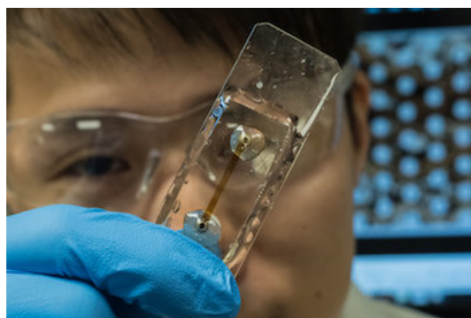
Graduate student Yu-Jiun Lin holds a microfluidic device used to show how and why dispersants are able to break up deposits of asphaltene that hinder the flow of crude oil in wellheads and pipelines. Credit: Jeff Fitlow/Rice University
