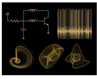
Chaotic voltage changes are common even for electronic circuits made up of only several elements. In the top left corner is a diagram of the simplest chaotic oscillator found by physicists from IFJ PAN in Cracow. On the right, a series of pulses showing a great resemblance to neural activity, generated by one of the newly discovered circuits. In the lower row several so-called attractors, illustrating the complexity of behaviour of the new circuits. Credit: IFJ PAN
