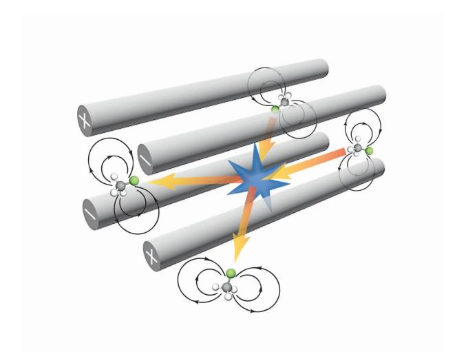
Schematic representation of cold collisions between polar molecules in a quadrupole guide. Credit: MPQ, Quantum Dynamics Division
