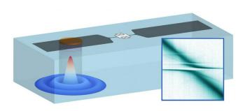
A schematic drawing of a superconducting qubit coupled to phonons inside a sapphire crystal. Inset shows the energy spectrum of phonons measured using the qubit. Credit: Yale University
