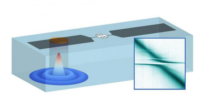
A schematic drawing of a superconducting qubit coupled to phonons inside a sapphire crystal. Inset shows the energy spectrum of phonons measured using the qubit. Credit: Yale University
