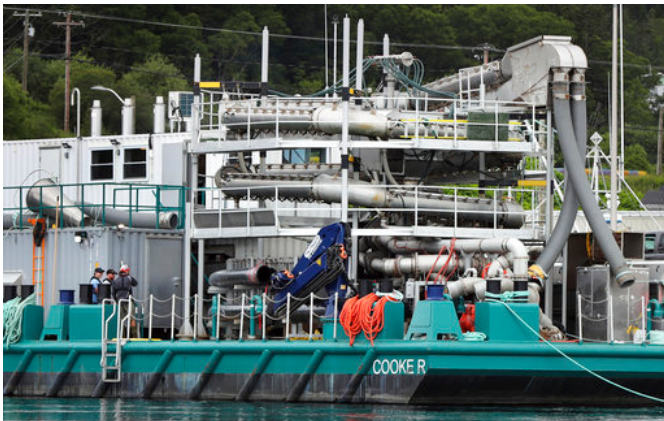
In this Thursday, July 13, 2017 photo, workers confer aboard a warm water lice removal vessel on Beaver Harbour in New Brunswick, Canada. The barge contains a series of tubes that send about 300 salmon a minute on a winding journey while dousing them with warm water to remove lice. The "waterslide park for fish" is one of the innovations being tested in the salmon farming industry's war against sea lice. (AP Photo/Robert F. Bukaty)
