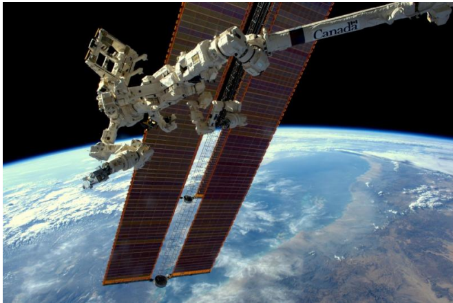
The Robotic External Leak Locator on the end of the Dextre robot in February 2017. Credit: NASA
