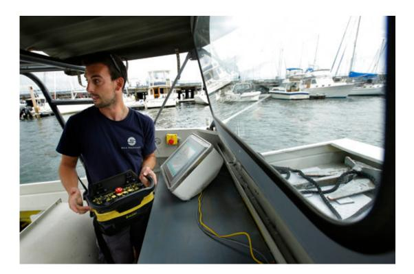
In this Aug. 15, 2017 photo, Frank Marino, an engineer with Sea Machines Robotics, uses a remote control belt pack to control a self-driving boat in Boston Harbor. Spurred on by the car industry's race to build driverless vehicles, maritime companies are taking advantage of technological breakthroughs and broader public acceptance of artificial intelligence to design tugboats, ferries and cargo vessels that won't need captains or crews, at least not on board. (AP Photo/Steven Senne)
