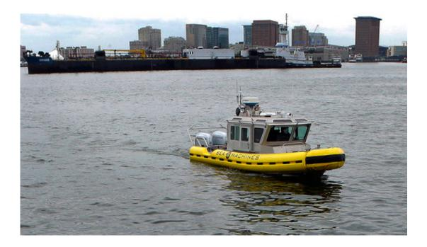
In this Tuesday, Aug. 15, 2017 photo, a boat capable of autonomous navigation makes its way around Boston Harbor. The experimental workboat spent this summer dodging tall ships and tankers, outfitted with sensors and self-navigating software and emblazoned with the words "UNMANNED VESSEL" across its aluminum hull. (AP Photo/Steven Senne)
