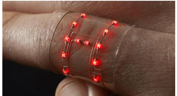
A hybrid 3D-printed device can repeatedly bend into a cylindrical shape without its LEDs failing. Credit: Wyss Institute for Biologically Inspired Engineering
