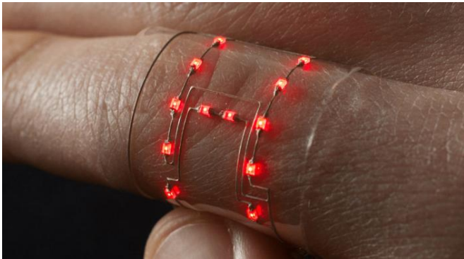
An array of silver-TPU ink sensors printed on a flexible TPU base. Credit: the Wyss Institute for Biologically Inspired Engineering
