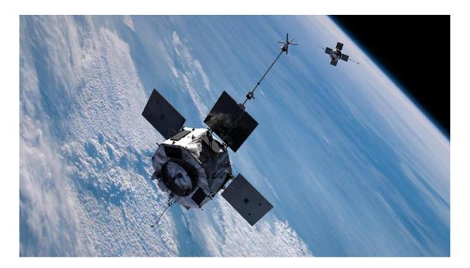
The two Van Allen Probes work as a team, following one behind the other to uniquely observe changes in the belts. Credit: NASA's Goddard Space Flight Center/JHUAPL
