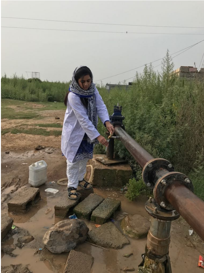
Collection of samples from a groundwater pump in the Gujrat district of Punjab province in Pakistan. Credit: Photo: Tasawar Khanam, COMSATS
