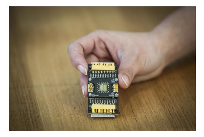
A semiconductor qubit device mounted on a custom cryogenic printed circuit board. Credit: Jayne Ion/University of Sydney, Author provided
