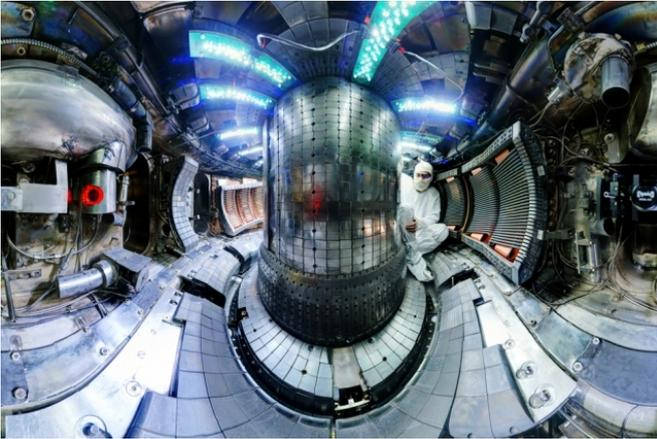
The interior of the Alcator C-Mod tokamak, where experiments were conducted that have helped create a new scenario for heating plasma and achieving fusion. Credit: Bob Mumgaard/Plasma Science and Fusion Center
