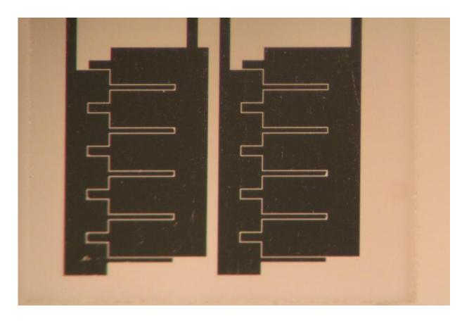
A close-up view of the lead sensor, featuring two pairs of electrodes. It could enable cities and homeowners to pinpoint pipes that taint water with lead. Credit: Wen-Chi Lin, Burns Lab, University of Michigan
