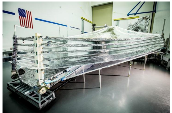
The first layer of the Webb telescope sunshield installed at Northrop Grumman's clean room in Redondo Beach, California. Credit: Northrop Grumman Corp.
