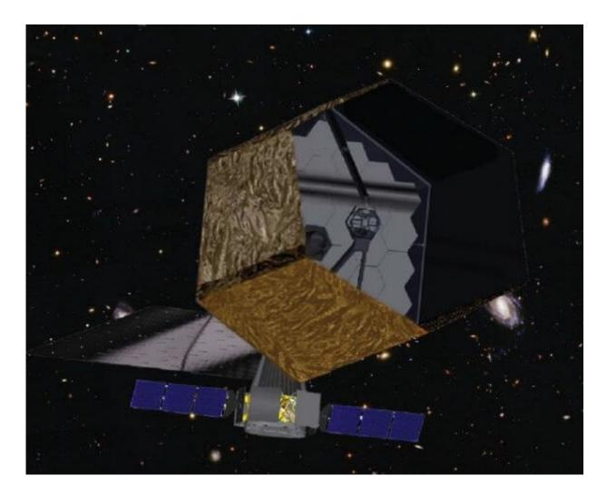
An artist's illustration of a 16 meter segmented mirror space telescope. There are no actual images of LUVOIR because the design hasn't been finalized yet. Credit: Northrop Grumman Aerospace Systems & NASA/STScI
