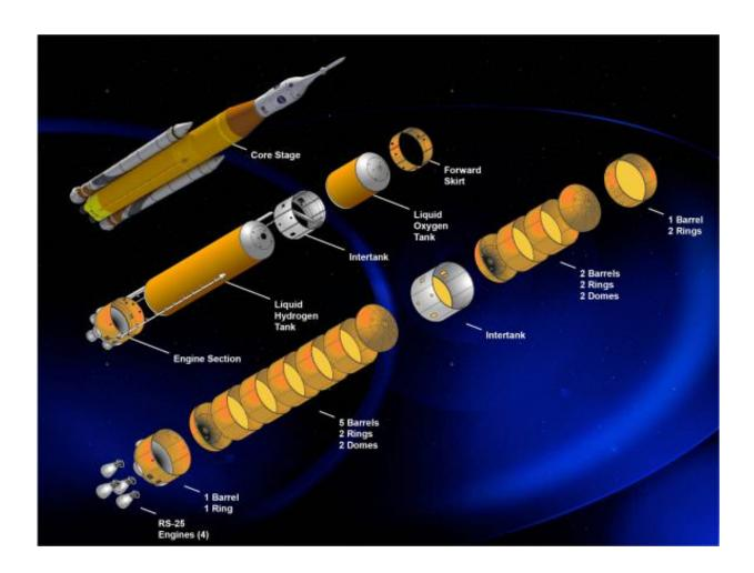
Graphic shows all the dome, barrel, ring and engine components used to assemble the five major structures of the core stage of NASA's Space Launch System (SLS) in Block 1 configuration. Credit: NASA/MSFC
