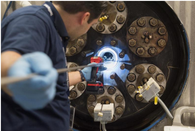
Kyle Phillips, NASA Glenn engineer, removes samples from GEER after they were exposed to Venus surface conditions for 80 days. Credit: NASA
