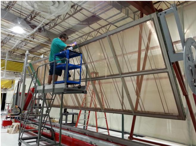
Physical Sciences Laboratory electronics technician Andy Arbuckle soldering 150 micron CuBe wire on the anode panel assembly (APA). Four underground detector modules in South Dakota will each be two-thirds the size of a football field and comprise 150 APAs. Credit: UW-Madison Physical Sciences Laboratory
