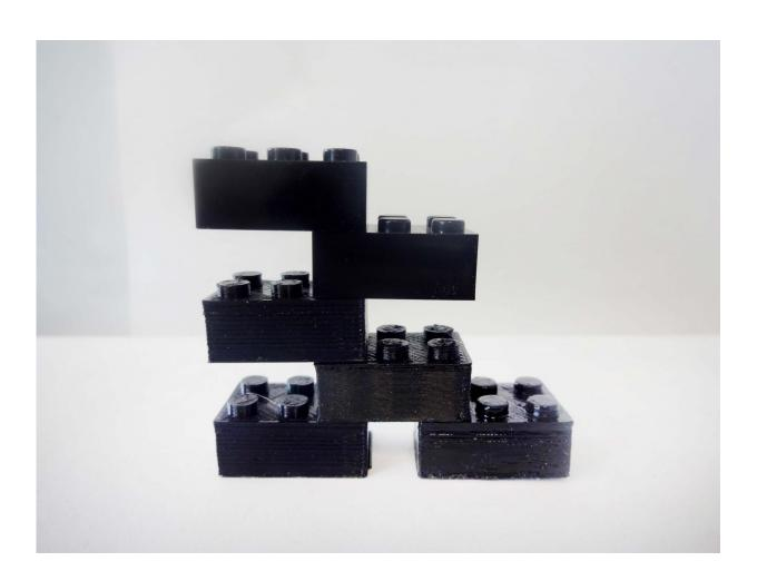
Each plastic building block is made of a different plastic and process; 3-D printing has the potential to disrupt conventional toy production, making it cheaper to make toys at home. Credit: Joshua Pearce
