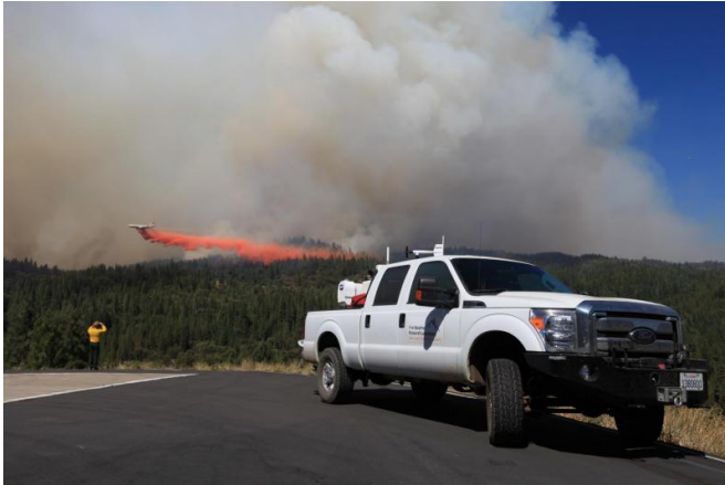
Doppler LiDAR is measuring winds near the plume of the King Fire in California in September, 2014. Credit: San Jose State University
