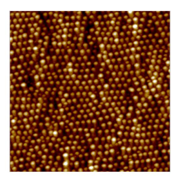
A microscopy photo showing an array of precisely placed metallic nanoparticles on the surface of a gallium arsenide semiconductor. Credit: Courtesy of Rachel S. Goldman, Michigan Engineering
