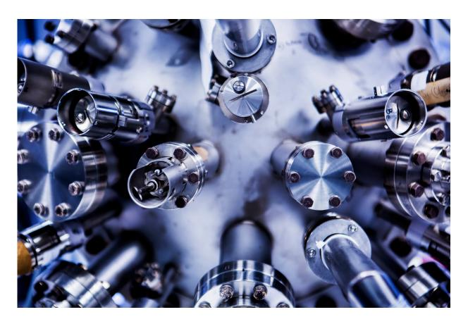
The main growth chamber of the molecular epitaxy beam apparatus used to make the nanoparticle-infused gallium nitride semiconductors. The semiconductors could boost LED efficiency by up to 50 percent, and even lead to invisibility cloaking devices. Credit: Photo by Joseph Xu, Michigan Engineering Communications & Marketing
