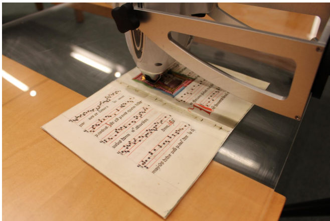
A portable-point X-ray fluorescence (p-XRF) scanner is used on an illuminated manuscript fragment. Credit: Cornell University Library
