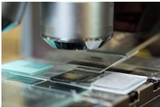
Samples produced by the meniscus-assisted solution printing (MASP) technique are studied under this optical microscope. Credit: Credit: Rob Felt, Georgia Tech
