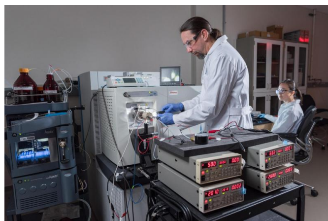
Research Scientist Alex Jonke (left) connects DRILL to a mass spectrometer in the Torres laboratory at Georgia
