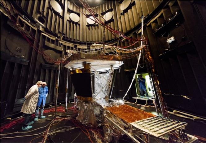
The solar array cooling system for the Parker Solar Probe spacecraft is shown undergoing thermal testing at NASA Goddard Space Flight Center in Greenbelt, Maryland, in late February. Credit: NASA/JHUAPL
