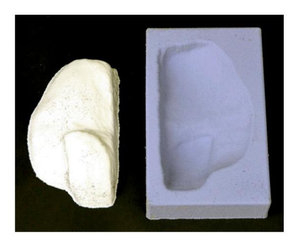
In this April 12, 2016 photo provided by Dartmouth College, a completed climbing hold, left, lies alongside its casting mold in Hanover, N.H. The hold, created by using three-dimensional geometry, is part of a replica of a rock wall created by tracking a climber's hand and foot positions and by estimating the contact forces. (Emily Whiting/Dartmouth College via AP)
