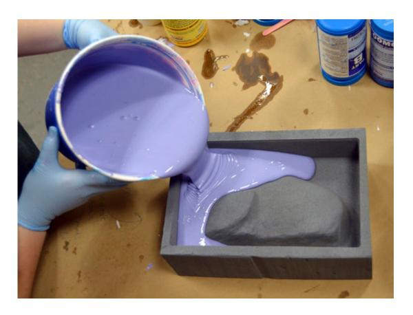
In this April 12, 2016 photo provided by Dartmouth College, silicone rubber is poured over a foam cast, created by using three-dimensional geometry, to create a mold for a hold that will be mounted on a climbing wall in Hanover, N.H. The hold, created by using three-dimensional geometry, is part of a replica of a rock wall created by tracking a climber's hand and foot positions and by estimating the contact forces. (Emily Whiting/Dartmouth College via AP)
