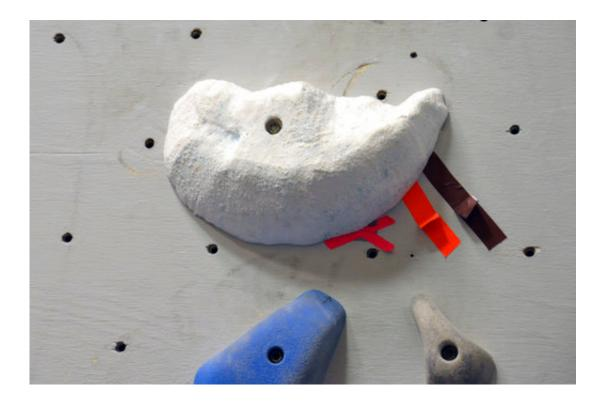
This Jan. 16, 2016 photo provided by Dartmouth College shows fabricated holds mounted on a climbing wall in Hanover, N.H. The hold, created by using three-dimensional geometry, is part of a replica of a rock wall created by tracking a climber's hand and foot positions and by estimating the contact forces. (Christos Mousas/Dartmouth College via AP)
