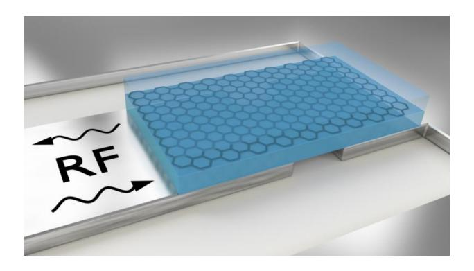
The layer of graphene (black honeycomb structure) encapsulated in boron nitride (blue) is placed on a superconductor (gray) and coupled with a microwave resonator. By comparing microwave signals (RF), the resistance and quantum capacitance of the embedded graphene can be determined. Credit: University of Basel, Department of Physics/Swiss Nanoscience Institute
