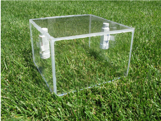
Litvak's mini-chamber was used to measure ET in urban lawns. Credit: Elizaveta Litvak
