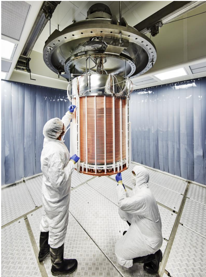
Scientists assembling the XENON1T time projection chamber. Credit: Enrico Sacchetti
