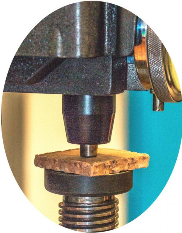
The ModRoof precursor material is tested for its structural integrity in a UC Berkeley engineering lab. Credit: Ryan Forster
