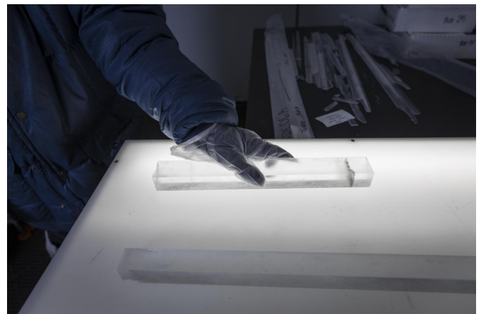
Close-up of an ice core from Antarctica with a darker layer of volcanic ash. The UW group is now analyzing these samples to see if they show the same trend as the Greenland cores. Credit: Mark Stone/University of Washington
