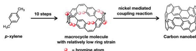
Figure 3. Synthetic approach towards the carbon nanobelt from p-xylene in 11 steps. Credit: Nagoya University
