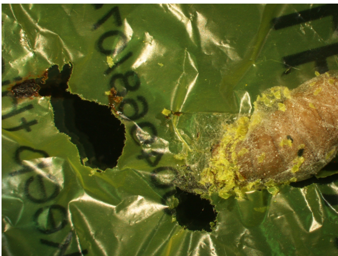
A close-up of wax worm next to biodegraded holes in a polyethylene plastic shopping bag from a UK supermarket as used in the experiment. Credit: Paolo Bombelli
