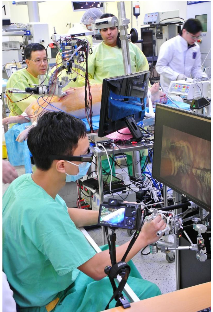
The robotic arms are highly sensitive to touch, have up to ten degrees of movement, and can perform surgical procedures by means of a single incision. Credit: The Hong Kong Polytechnic University
