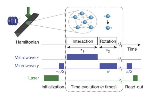
Observation of discrete time-crystalline order in a disordered dipolar many-body system. Nitrogen–vacancy centres (blue spheres) in a nanobeam fabricated from black diamond are illuminated by a focused green laser beam and irradiated by a microwave source. Credit: (c) *Nature* (2017). DOI: 10.1038/nature21426
