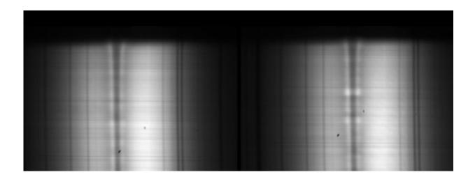
A first-light image from CryoNIRSP. It delivers two spectra simultaneously with opposite polarizations (the left and right panels above). This image shows light from near the edge of the Sun spread out horizontally in wavelength, near the wavelength of a prominent absorption line of Calcium. Credit: UH Institute for Astronomy
