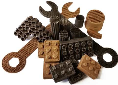
Tools and building blocks made by 3D printing with lunar and Martian dust. Credit: Northwestern University
