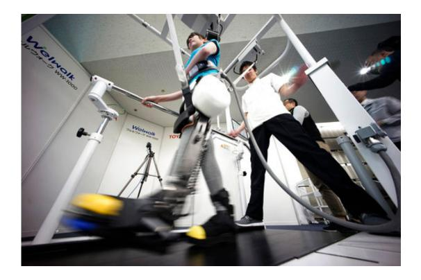
A model demonstrates the Welwalk WW-1000, a wearable robotic leg brace designed to help partially paralyzed people walk at the main system with treadmill and monitor, at Toyota Motor Corp.'s head office in Tokyo, Wednesday, April 12, 2017. Toyota Motor Corp.'s Welwalk WW-1000 system is made up of a motorized mechanical frame that fits on a person's leg from the knee down. (AP Photo/Eugene Hoshiko)
