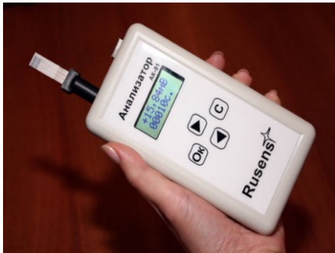
A chemical sensor on the basis of materials possessing molecular memory. Credit: Vita Nikitina
