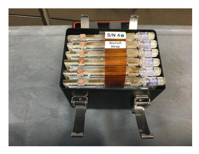
The Plate Habitat (PHAB) containing BioCell cassettes for the Expanded Stem Cell investigation aboard the space station. Credit: BioServe Inc., University of Colorado
