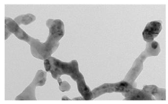
20 nanometer double perovskite nanofiber that can be used as a highly efficient catalyst in ultrafast oxygen evolution reactions -- one of the underlying electrochemical processes in hydrogen-based energy and the newer metal-air batteries. Credit: Georgia Tech
