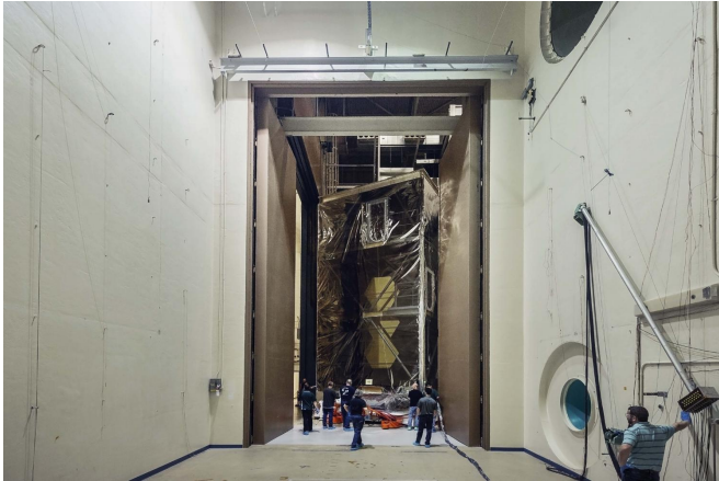
The James Webb Space Telescope inside the acoustics chamber at NASA's Goddard Space Flight Center in Greenbelt, Md. Credit: NASA
