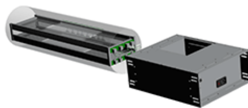
Prototype of the borehole-sized muon detector. Credit: Pacific Northwest National Laboratory
