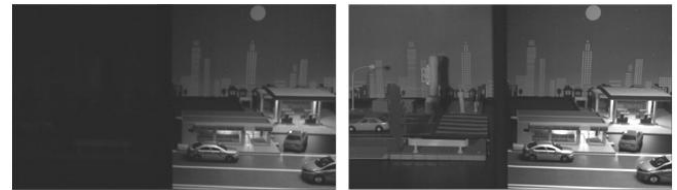
Fig.2. Images captured in color imaging mode (Left) and NIR imaging mode (Right).
