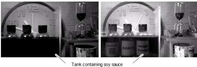
Fig.3. Images captured in color imaging mode (Left) and NIR imaging mode (Right). NIR imaging makes it possible to see characters on the labels of small bottles over a tank filled with soy source.
