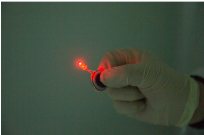
This is a coin-shaped seawater battery, developed by Professor Youngsik Kim's research team at UNIST. Credit: UNIST
