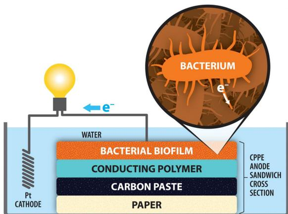
A schematic illustration of a microbial fuel cell using a paper electrode coated with carbon paste. Credit: Michael Osadciw/University of Rochester
