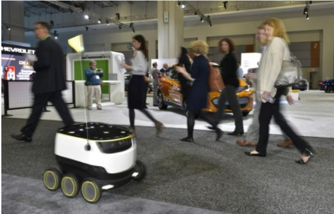
The goal for Starship Technologies robots is to carry about nine kilograms of goods within a radius of three kilometres for \$1 or less
